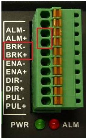
To operate the motor, the brake must be supplied with 24V. If the brake is not supplied with the correct voltage (24V) and sufficient current (150mA), it is fixed. It is strongly recommended not to operate the motor with the brake fixed, as the increased current consumption can damage the electronics.
