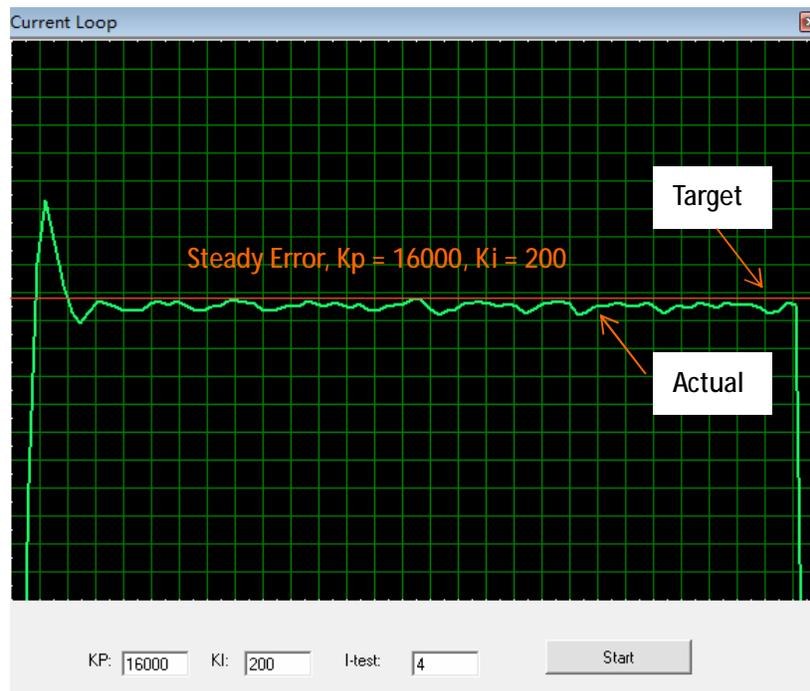
The current loop tuning is basically finished now. You can continue to adjust the  $K_p$  and the  $K_i$  if necessary.
