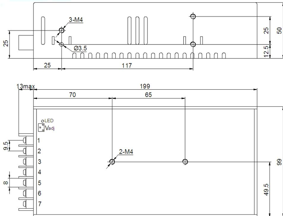
**Length of assembly screw: max. 6mm**
